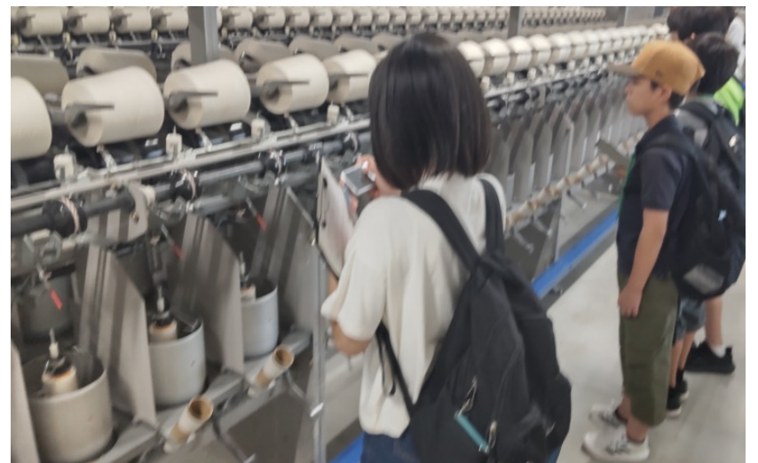
The twisting machines in the factory at Asano Nenshi's Futaba Plant
