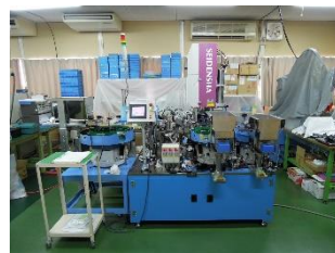
Automatic assembly machine for PV connectors
